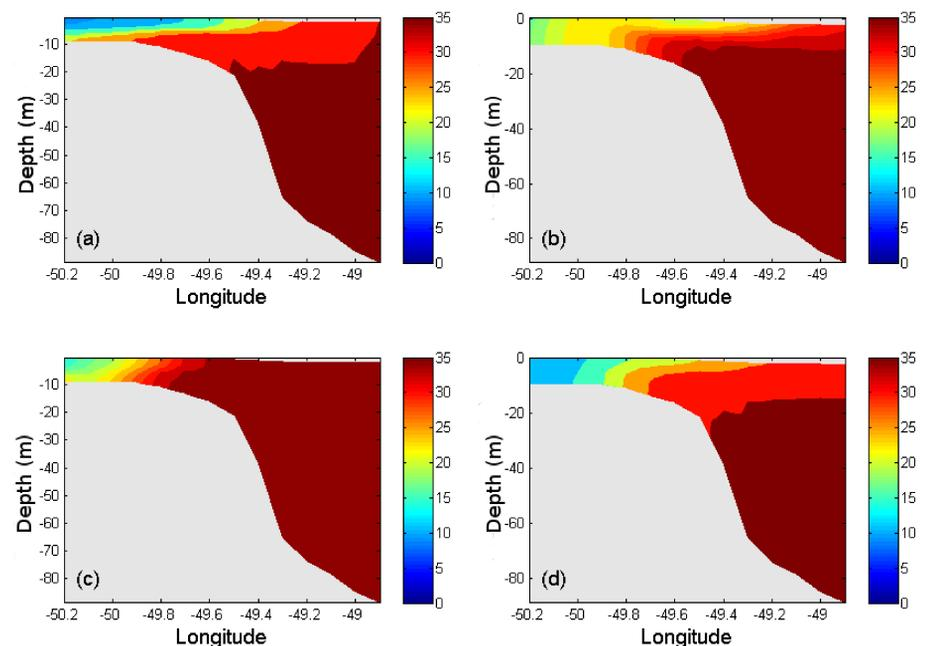
Figure 3: Vertical profiles at PII; Monthly composed average salinity during (a) high river runoff in experiment one; (b) high river runoff in experiment two; (c) low river runoff in experiment one; (d) low river runoff in experiment two.
